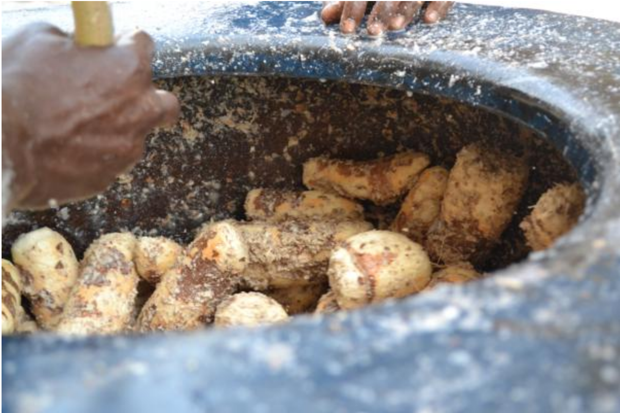
Figure 7: Motorised peeling machine. Wahan Foods Ltd., Kwara State
