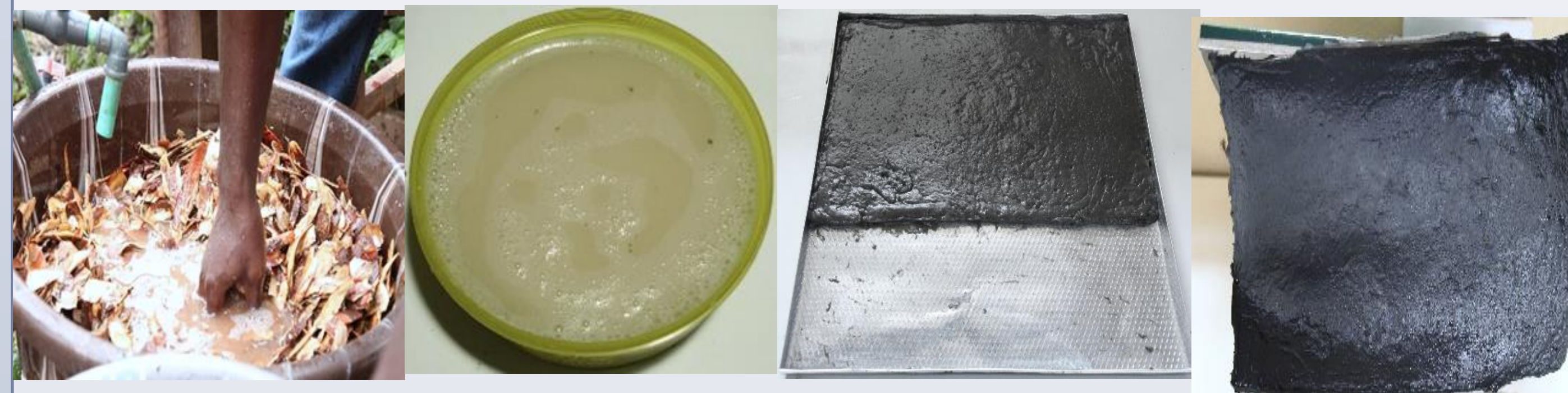
Cassava Peels Starch from Peels Bio-resin (PFA) Bioplastic
