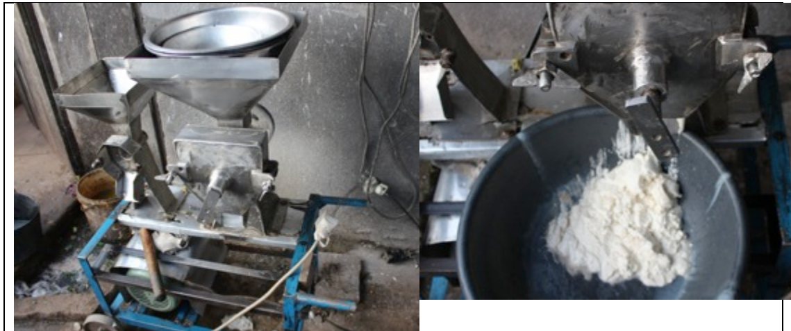
Example of a multi purpose cassava crusher/paster. Oyem main market.
