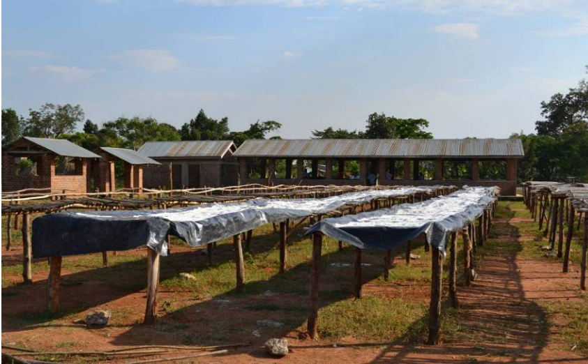
Figure 30: Small scale sun drying racks in series, and behind, typical village scale cassava processing structure
