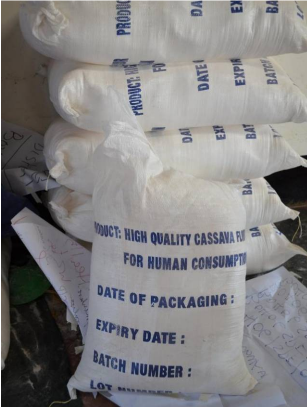
Figure 24: Correct bagging of flour with PE lined PP bags
