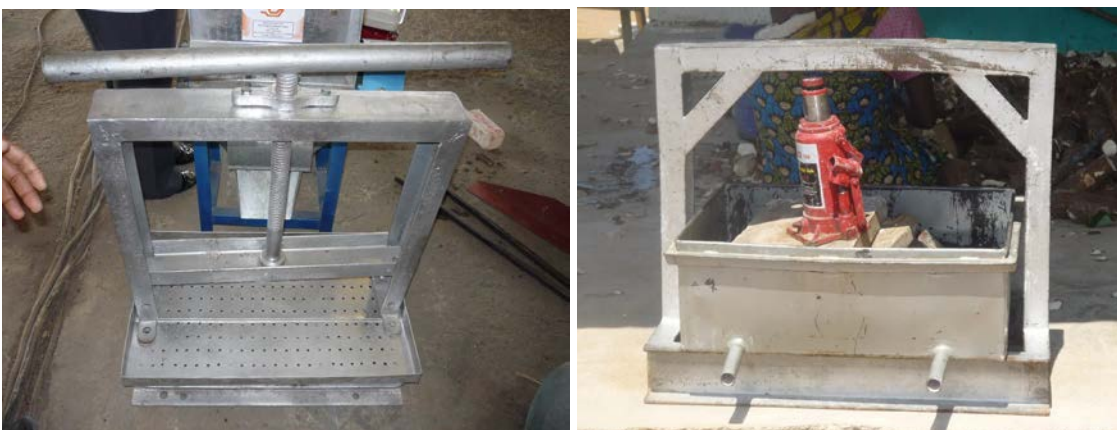
Figure 15: Household (low capacity screw) dewatering press
