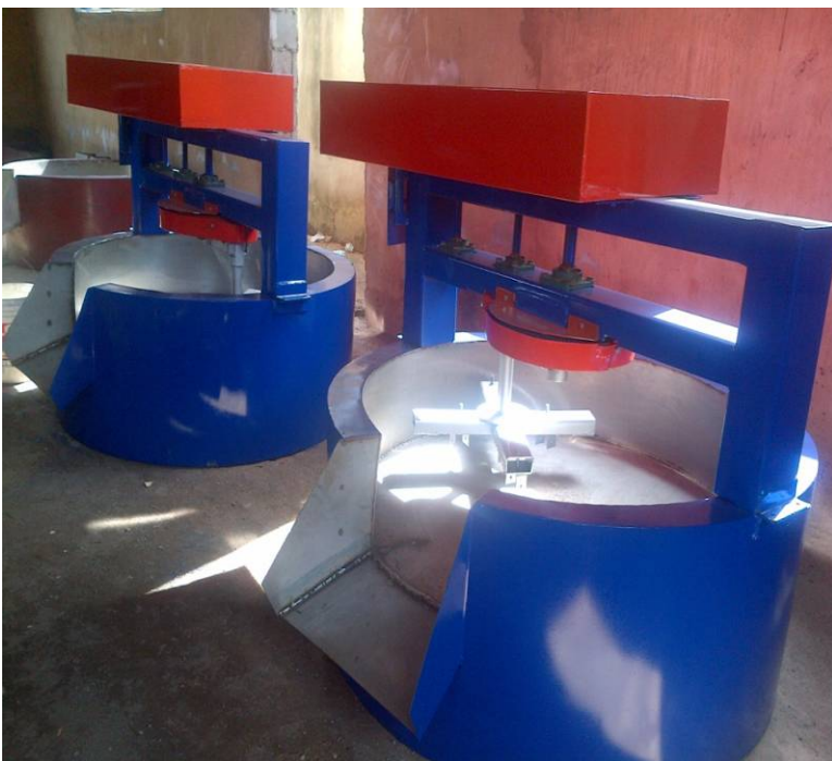
Figure 22: Semi-automated gari fryer for processing larger batches
