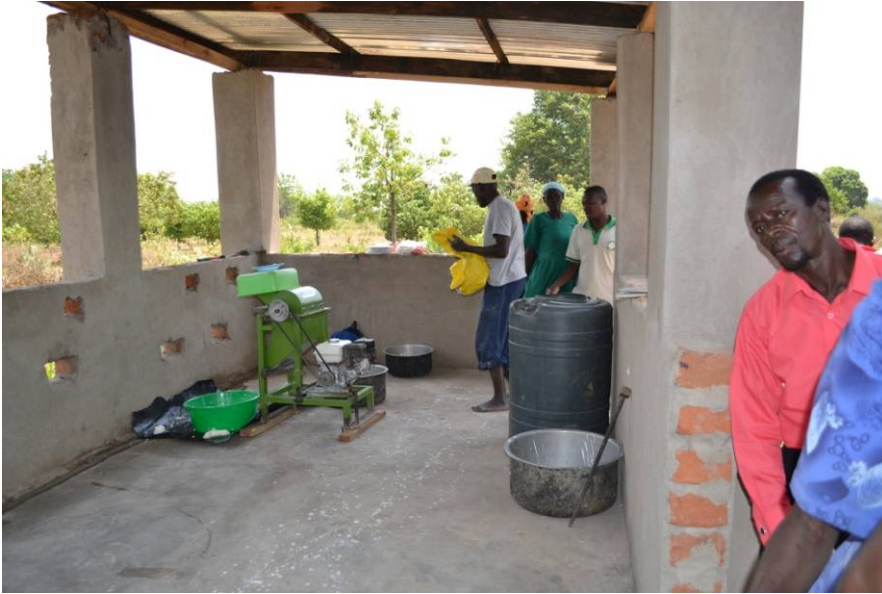
Figure 28: Simple processing plant showing wet processing (grating) carried out
