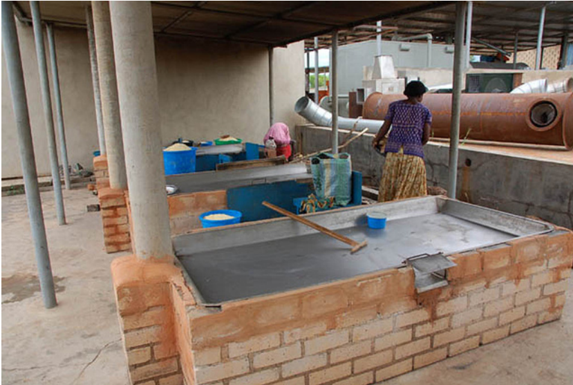
Upgraded gari frying layout showing multiple frying units
