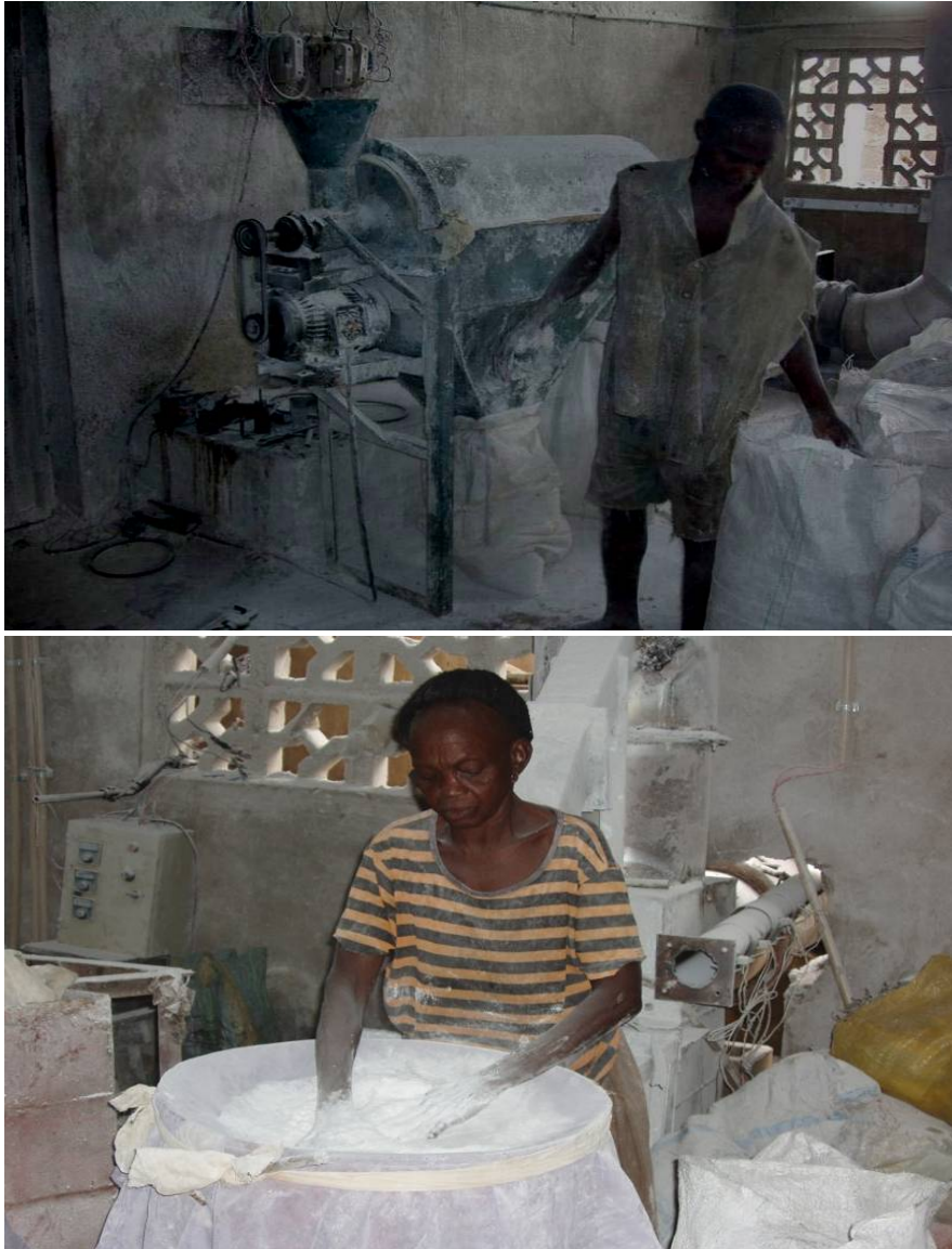
Figure 23: Small scale milling and screening of dried cassava grits
