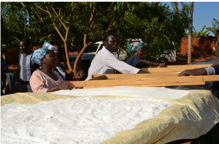
Figure 20: Parallel screening and spreading of wet cake for drying
