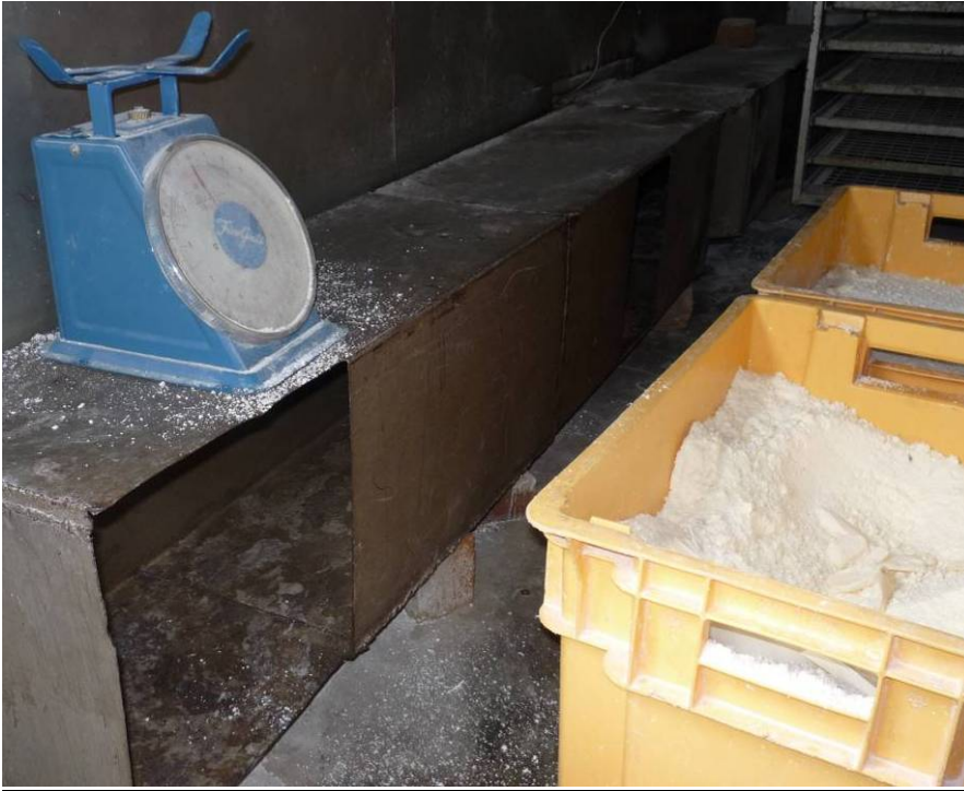
Figure 17: Resultant cassava screened wet cake in containers awaiting frying (gari) or drying (HQCF)
